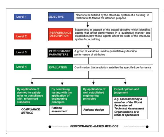
1 The performance framework for the design and appraisal of a structural system for a building to satisfy fitness for purpose requirements (after Watermeyer and Milford, 2003)
